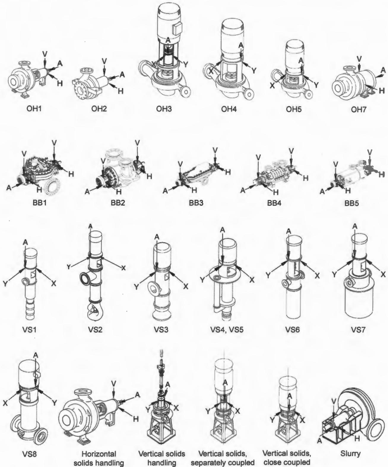
**Figure 9.6.4.2.3.1 — Measurement locations and directions (For a more complete description of pump types, refer to ANSI/HI 1.1-1.2 and ANSI/HI 2.1-2.2.)**
