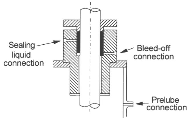
Figure A.7 — Packed-type stuffing box
