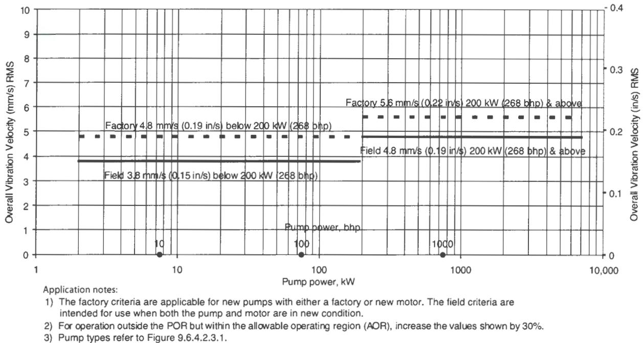
**Figure 9.6.4.2.5.1a — Allowable pump vibration, pump types BB and OH** (For a more complete description of pump types, refer to ANSI/HI 1.1-1.2 and ANSI/HI 2.1-2.2.)
