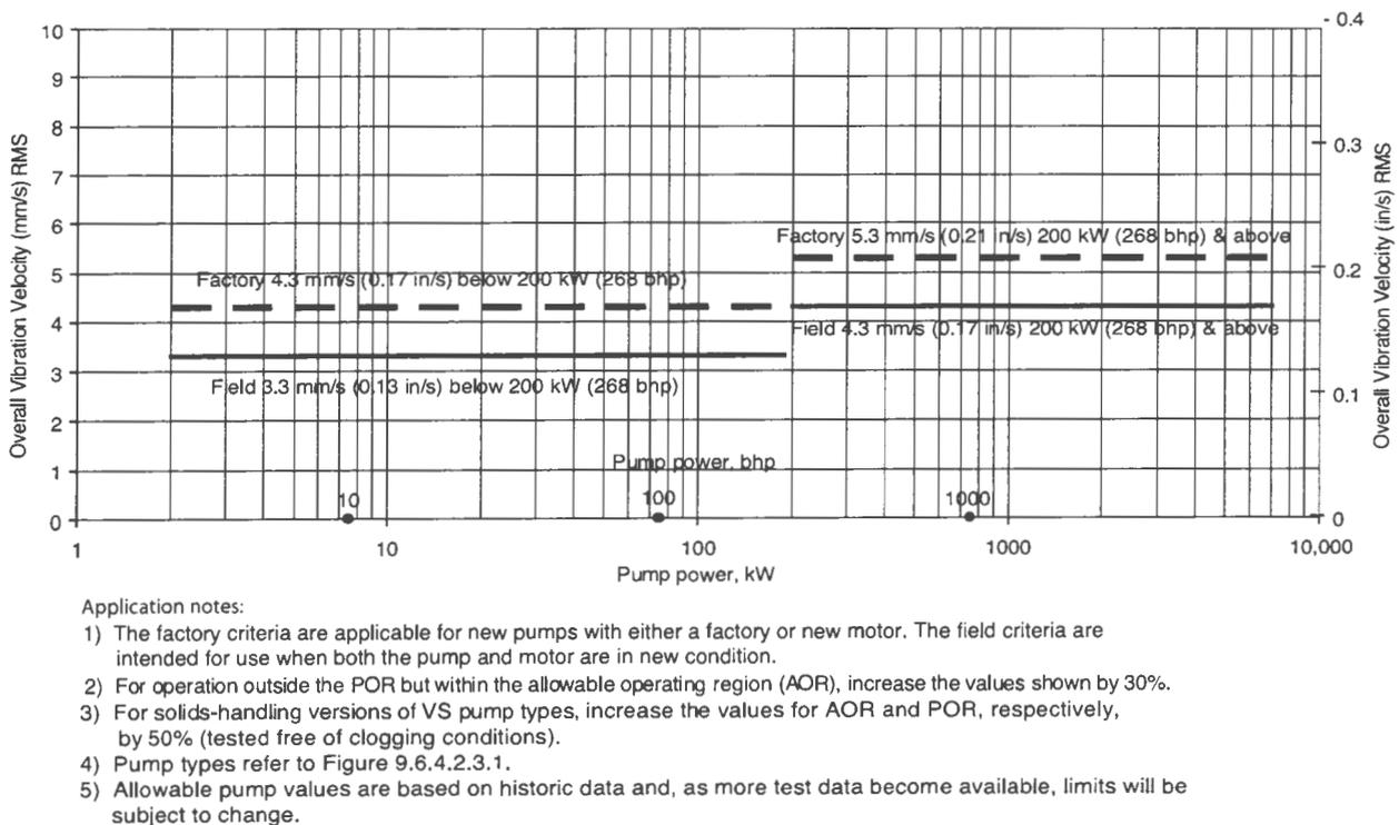
**Figure 9.6.4.2.5.1b — Allowable pump vibration, pump types VS1, VS2, VS3, VS4, VS5, VS6, VS7, and VS8** (For a more complete description of pump types, refer to ANSI/HI 1.1-1.2 and ANSI/HI 2.1-2.2.)
