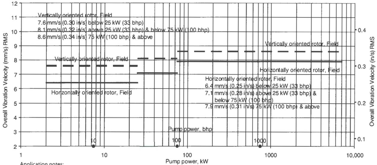
Figure 9.6.4.2.5.1c — Allowable pump vibration, solids-handling pump types
