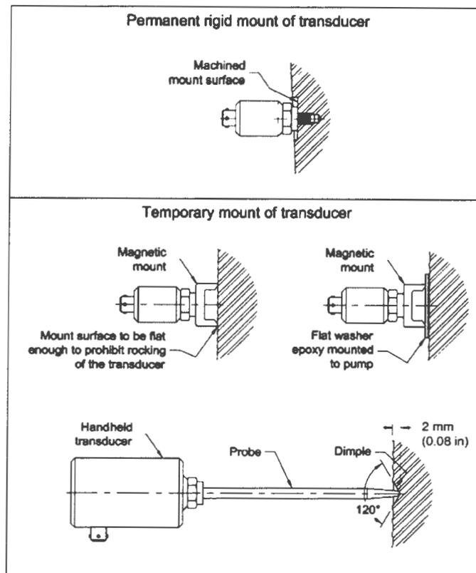
Figure 9.6.4.2.2.2 — Mounting methods for vibration transducers
