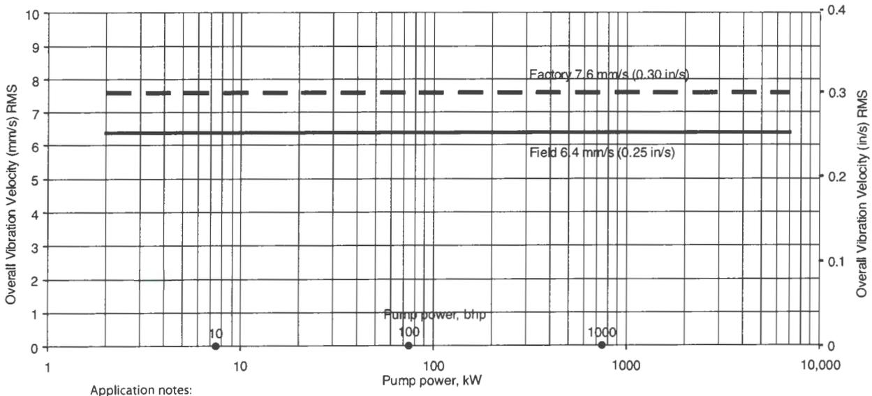
Figure 9.6.4.2.5.1d — Allowable pump vibration, horizontal and vertical slurry pump types (excluding wet pit cantilever belt-driven pumps with overhung motors)
