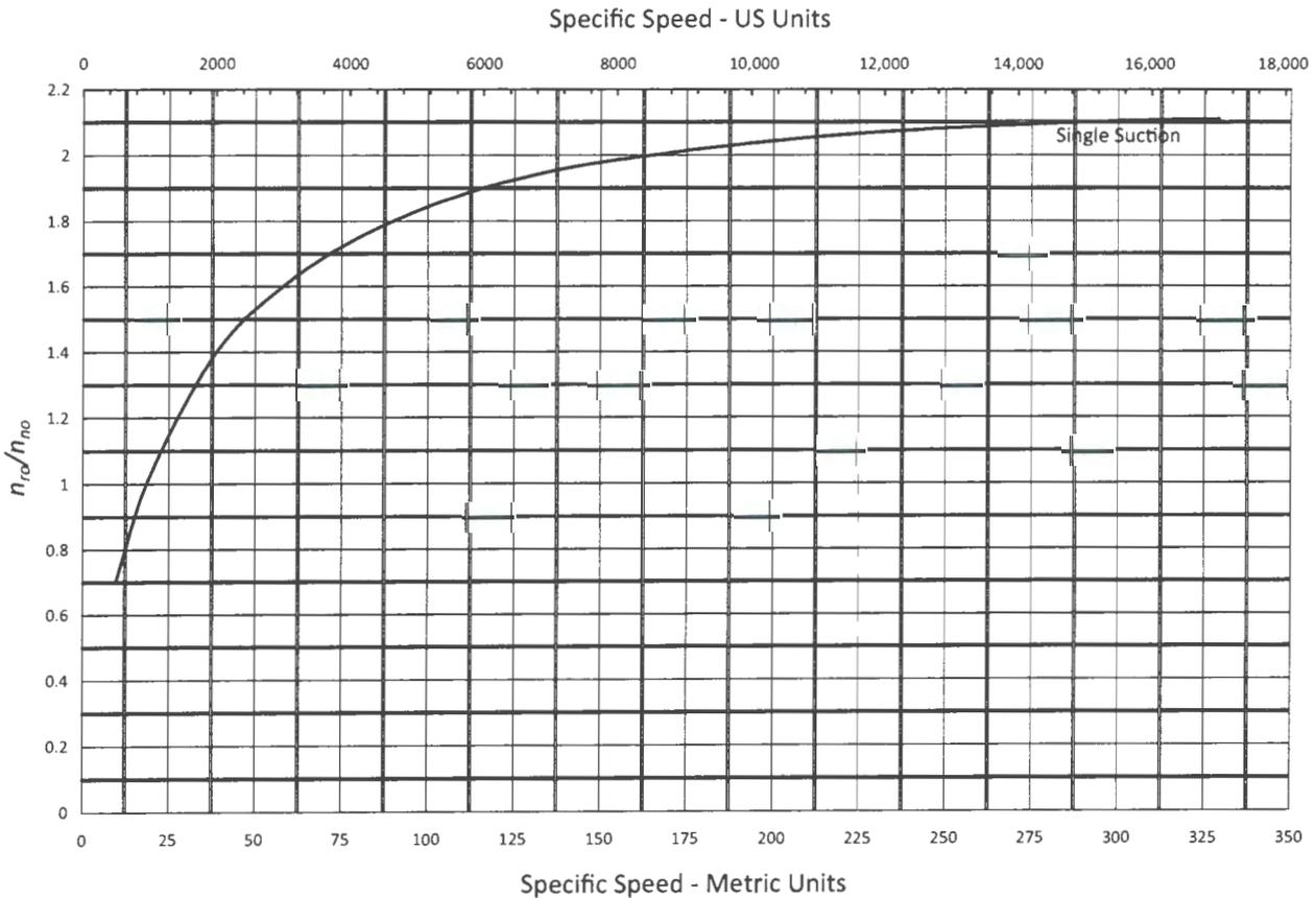
Figure A.6 — Reverse runaway speed ratio versus specific speed (metric and US customary units)
