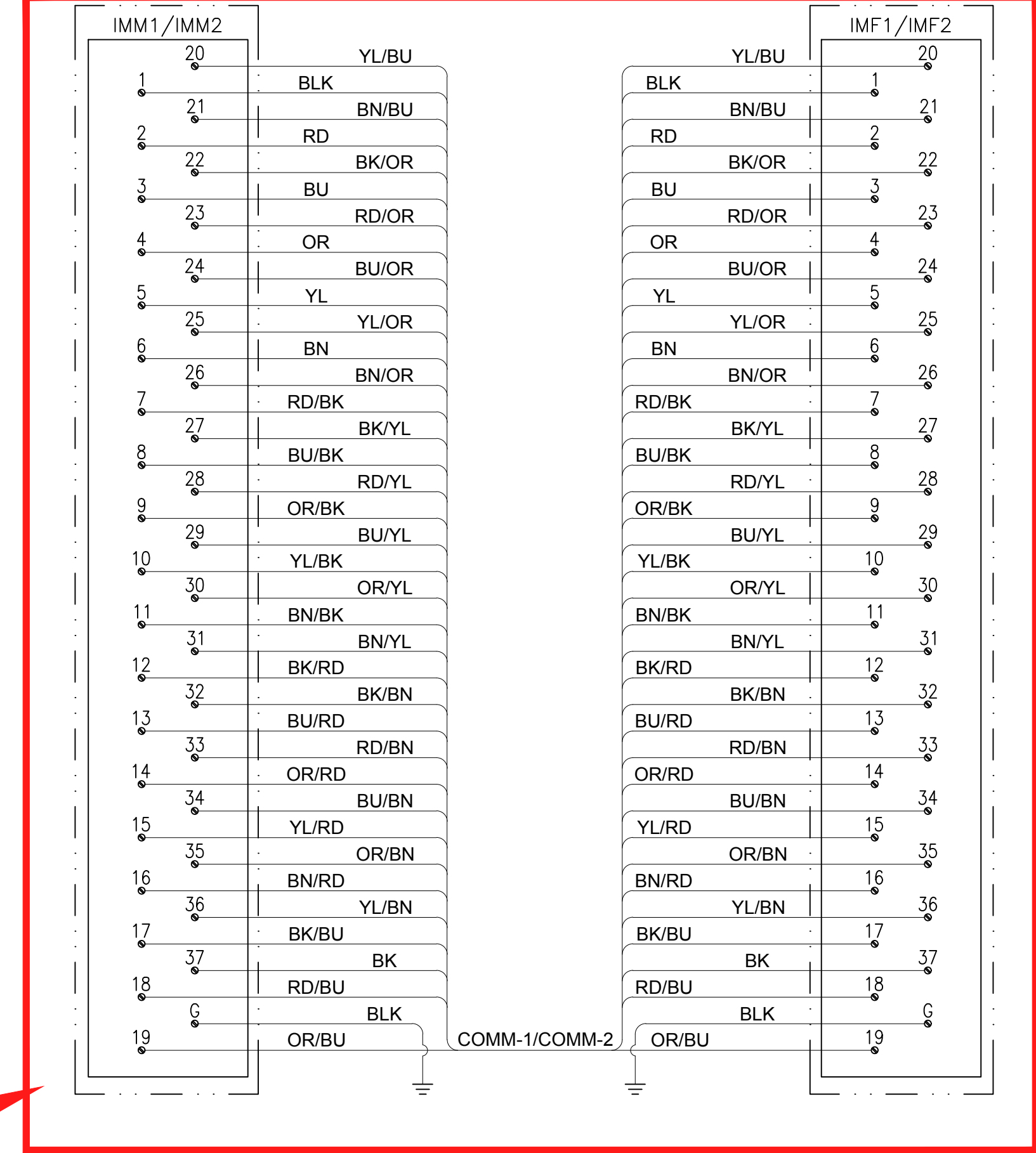
PUMP 1 PANEL/PUMP 2 PANEL *TYPICAL WIRING FOR BOTH SOFT STARTS
